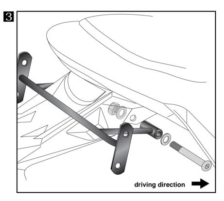
Fastening of the C-Bow: with hexagon bolts M6 x 16 and washers Ø6,4.
